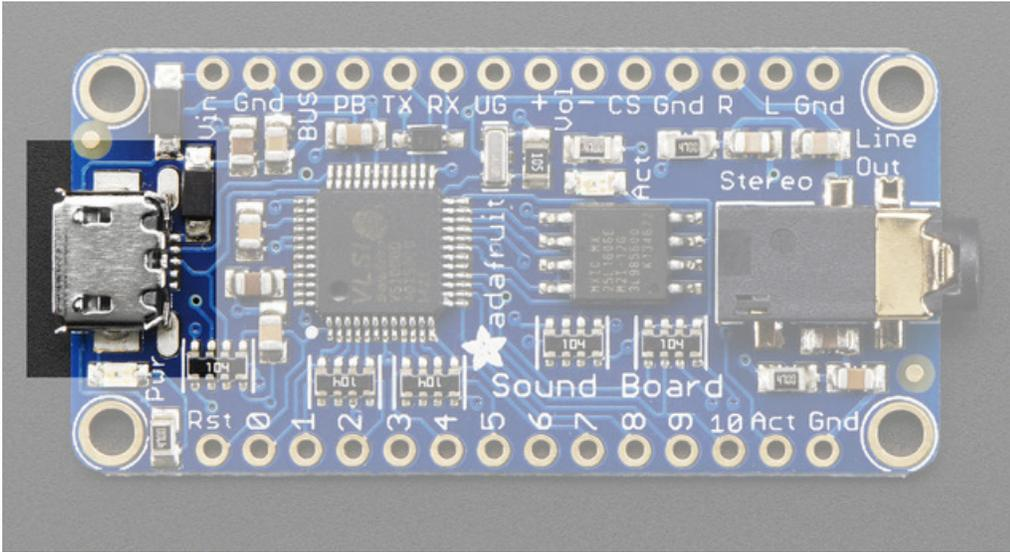
Starting from the left is the micro USB jack. You'll need a standard MicroUSB cable to connect this to your computer. You do need a computer (any will do) in order to save files onto the Sound Board flash storage
