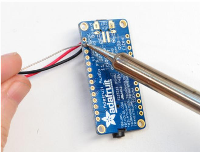
Solder both wires securely. You **cannot** just twist the wires into place!
