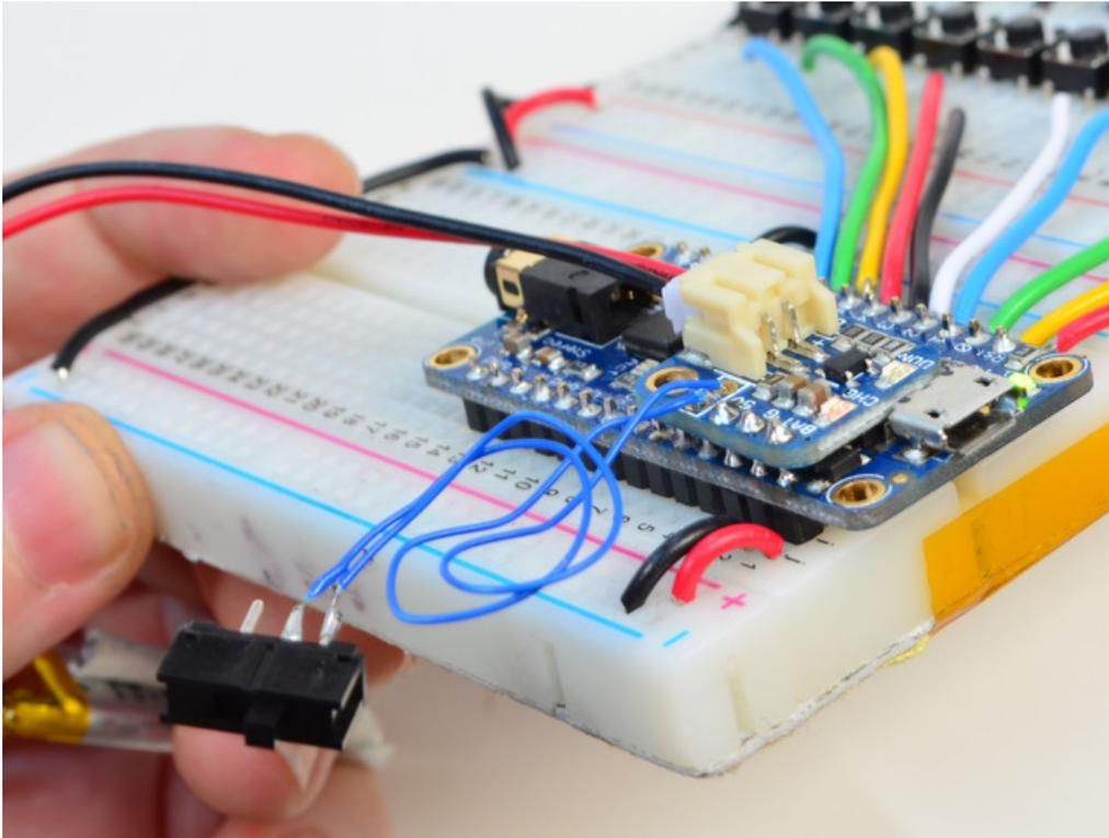
The Lipoly backpack lets you plug in a lipoly battery of any size and recharge it over the MicroUSB connector, so it's basically an all-in-one portable + rechargeable system.
