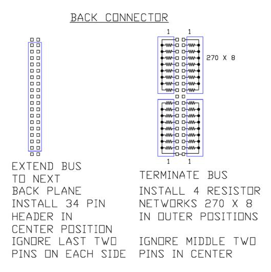
Extending the bus on high speed systems (over 4Mhz) might present a problem as the connectors between two backplanes may cause undesired reflections. It has not been tested but the option is there for your choice to try. No guarantees of performance are given. Perhaps one way to minimize the medium transition is to use PCB mounted ribbon cables (eg. Digikey Part number 1658525-2-ND) instead of pin headers with connectors & ribbon cables.
