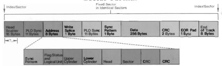
Typical sector format showing separate header and data fields with check codes for high reliability and data security.
