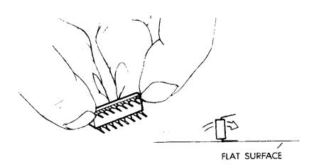
HOLDING EACH SIDE OF THE CHIP FIRMLY AGAINST THE FLAT SURFACE WITH BOTH HANDS, ROTATE IT A SHORT DISTANCE UNTIL THE PINS ARE BENT PERPENDICULAR TO THE BODY.
