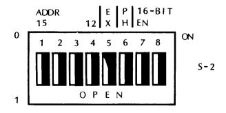
Extended addressing is shown "turned off" on S-2. The board now disregards any information conveyed by the extended address lines A-16 through A-23.
