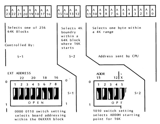
Extended addressing replaces the older bank select schemes which turn memory boards on and off through the use of an output port.
