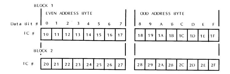
Normally, while running a program, memory cells are selected in sequence. If 16-bit transfers are being used, the program counter will step the memory address two bytes per increment (always using the even address). If 8-bit transfers are called for, the counter will increment the memory address one byte at a time.
