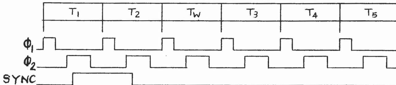
Dual-D flip flop U67 is used to set the number of wait cycles the CPU goes through when reading or writing data on this board. It signals that it is ready to read or write by actuating the Ready line (PREADY).
