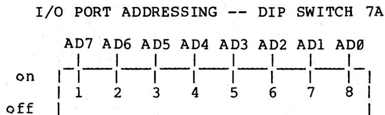
A paddle in the "off" position is to be taken as a cleared bit, while a paddle in the "on" position sets the bit. Thus, if all the paddles of the switch are turned to the "off" position, 0 would be the I/O port number assigned to the Memory Master board. When all the paddles of DIP switch 7A are in the "on" position, 255 (FF Hex or 377 Octal) is the I/O port number which is used to
