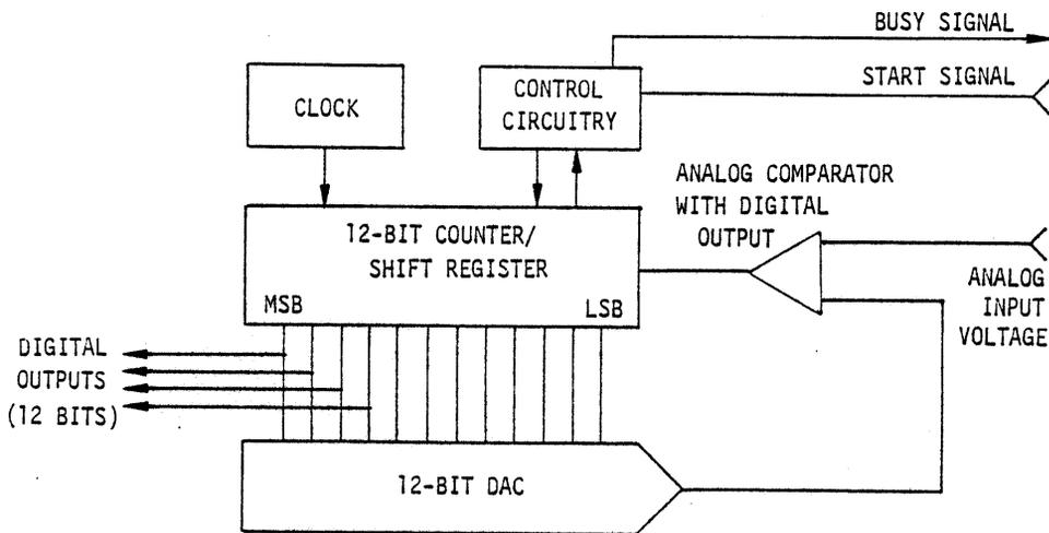
Figure 3-1. A/D Module Internal Block Diagram
