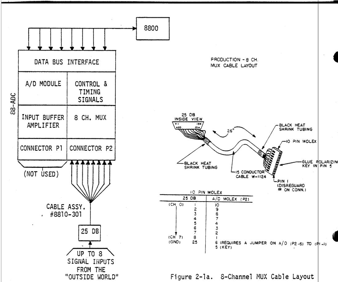
Figure 2-1a. 8-Channel MUX Cable Layout
