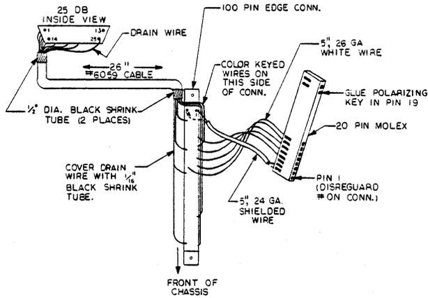
PRODUCTION MUX CABLE - 24 CHANNEL
