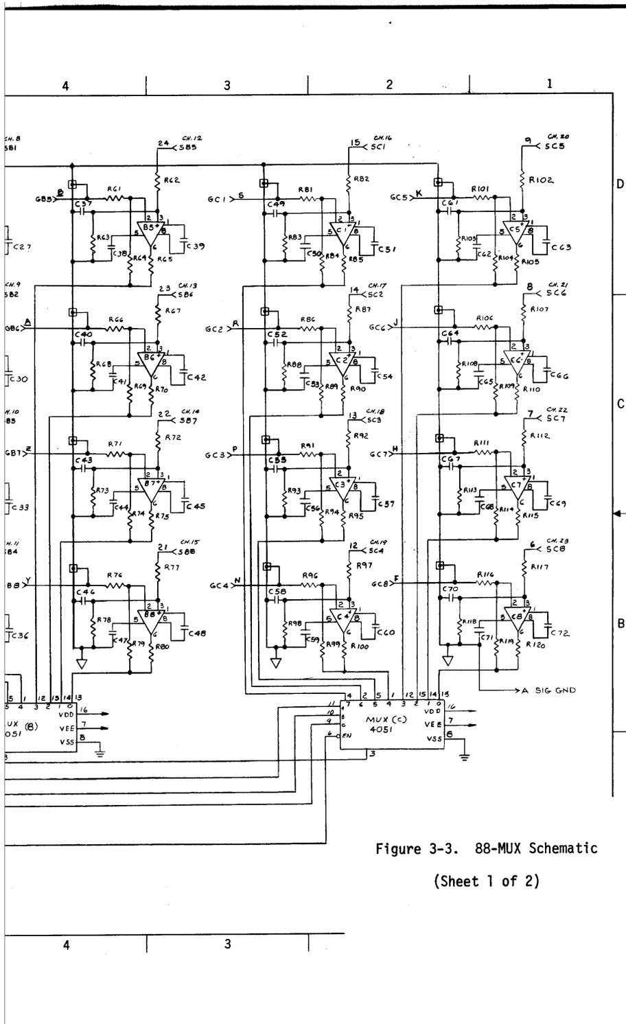
Figure 3-3. 88-MUX Schematic
