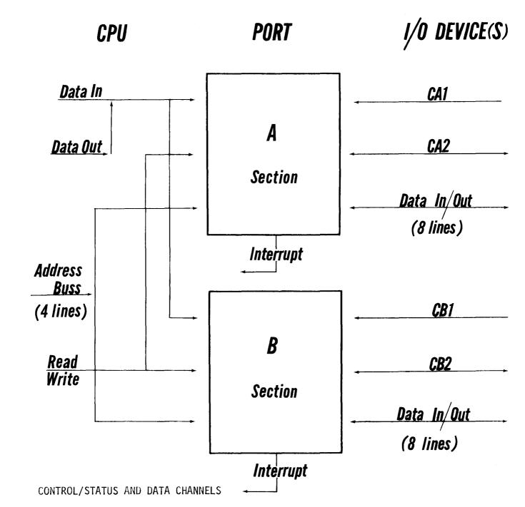
Each port section, A and B, contains three registers, eight data lines, two control lines and an interrupt request output. The control/status register, designed as follows, is a read/write register, meaning that it can be input from and output to.
