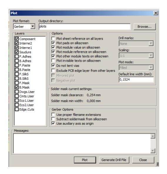
In these formats, a fine scale adjust can be used to compensate for the plotter accuracy and to have a true scale 1 for the output:
