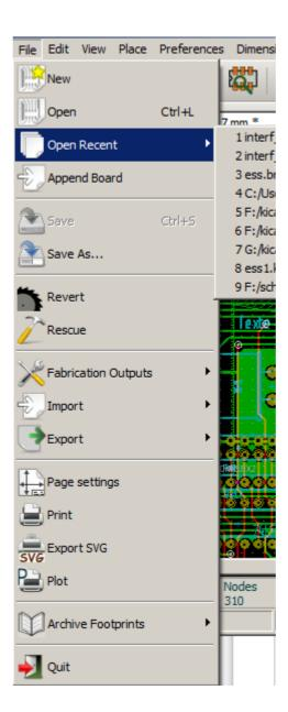
The File menu allows the loading and saving of printed circuits files, as well as printing and plotting the circuit board. It enables the export (with the format GenCAD 1.4) of the circuit for use with automatic testers.
