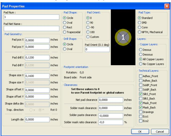
Care should be taken to define correctly the layers to which the pad will belong. In particular, although copper layers are easy to define, the management of non-copper layers (solder mask, solder pads...) is equally important for circuit manufacture and documentation.
