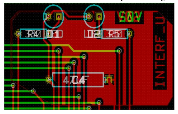
The polygon is the border of the filling area. You can see a non-filled area inside the zone, because this area is not accessible:
