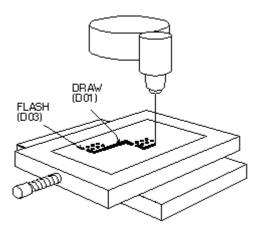
Figure 2. Plotter Operation
