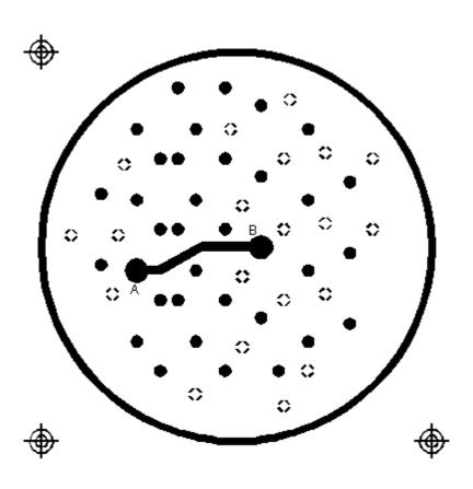
Internal\_VCC data. Note the large pads at A,B and the fat clearance trace.
