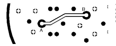
The dark VCC layer merged with the clear TRACE layer but before polarity reversal.
