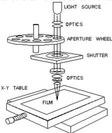
Figure 1 - Photoplotter Schematic
