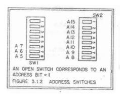
Next, the board address is selected. The lower address bits, A7-A5, are set with DIP switch SWI (for both 8-bit and 16-bit addressing) The upper address bits, A15-A8, (set only for 16 bit I/O addressing) are set with DIP switch SW2. See Figure 3.1.2.
