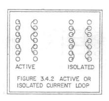
When a current loop circuit is being used, the activity of the current loop must be determined and set. The activity of the current loop circuit refers to whether the 6SIO provides the supply voltage and ground to the current loop (active loop), or the peripheral supplies the voltage and ground, and the current loop is opto-isolated from the rest of the 6SIO (isolated loop). Note that an active current loop pair must be connected to an isolated current loop pair and vice versa.
