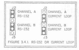
Current loop data transmission is used when electrical isolation is desired between interfacing devices. The current loop option is selected with jumpers J2 and J3 (Figure 3.4.1).
