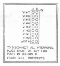
The interrupt controller on the 6SIO-1 generates an interrupt signal when programmed to do so. The 6SIO-Ø generates an interrupt signal in accordance to the configuration of header H3. This signal may be connected to the S-1ØØ pINT\* line or to any of the S-1ØØ VI\* lines Ø through 7 by positioning the shunt on jumper J5. The option should be set according to the system configuration. See Figure 3.6.1.
