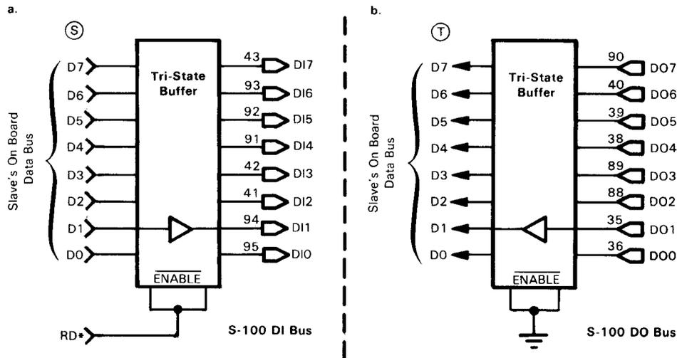
FIGURE 5-43. Data Bus Buffers for Unidirectional Buses
