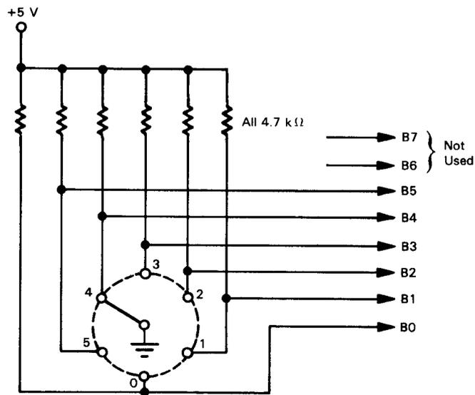
FIGURE 9-3. Connecting Rotary Switch to an Input Port
