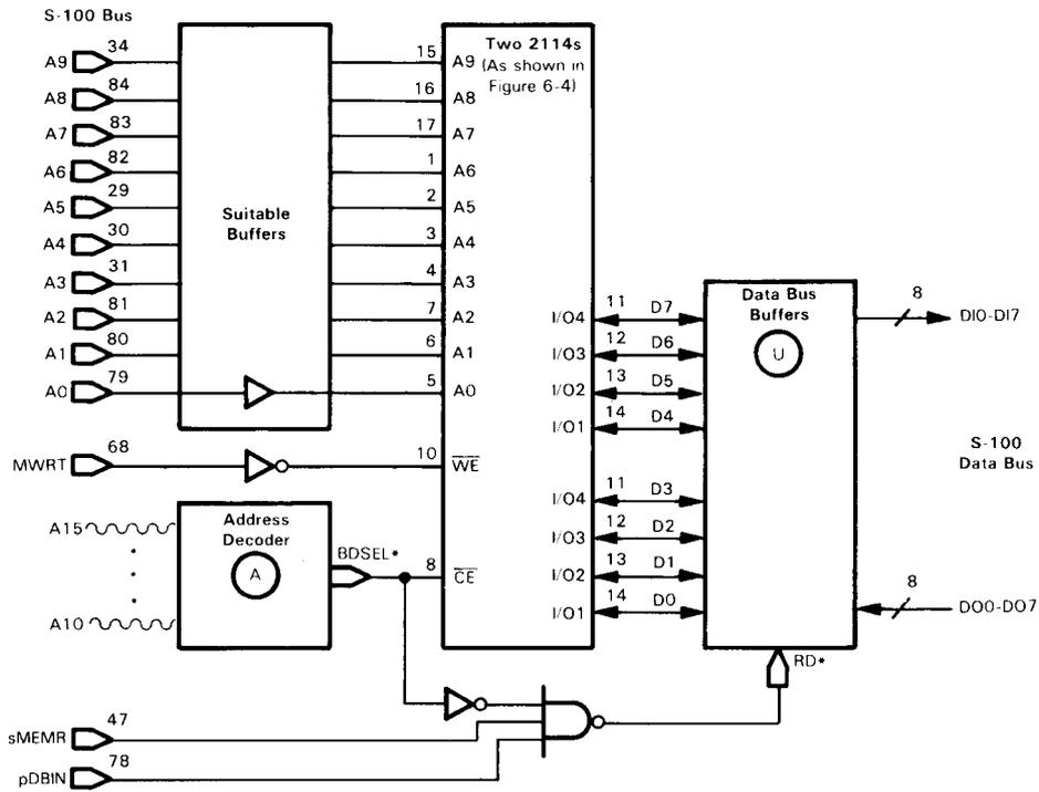
FIGURE 6-9. 1K × 8 of 2114-Type-Memory Interfaced to the S-100 Bus
