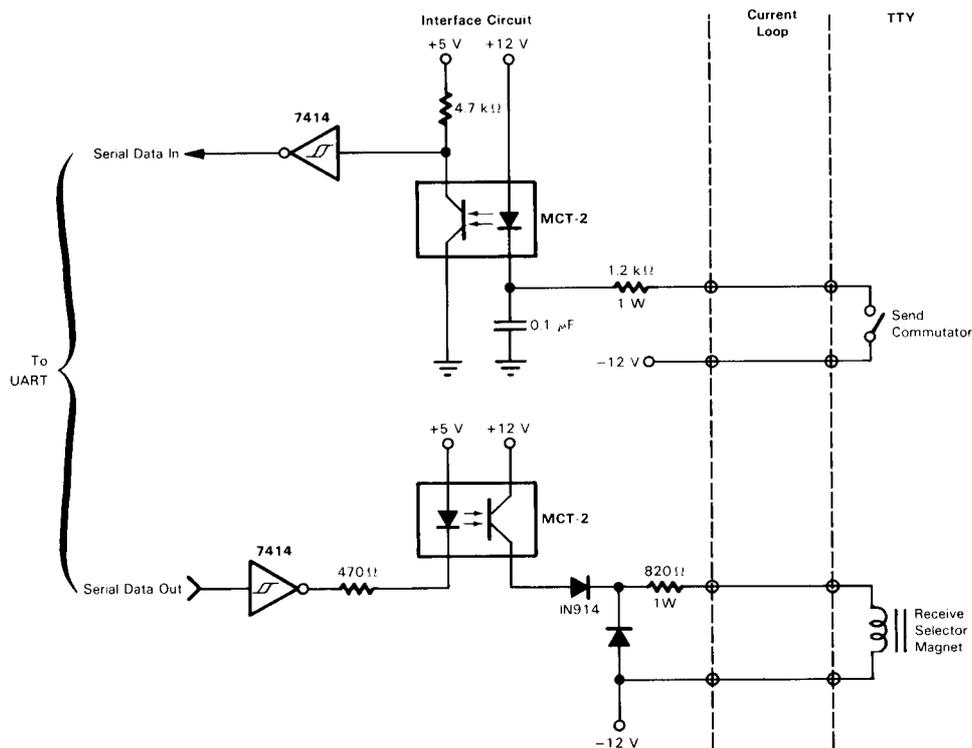
FIGURE 11-11. 20 mA Current Loop Interface Circuit
