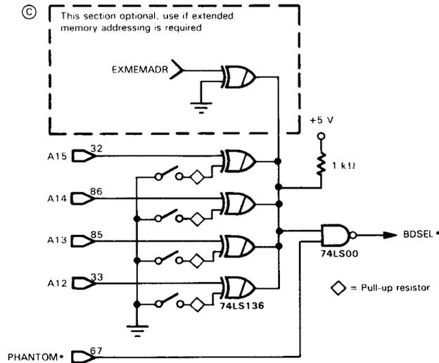
FIGURE 5-21. Memory Address Decoder for One 4K Block
