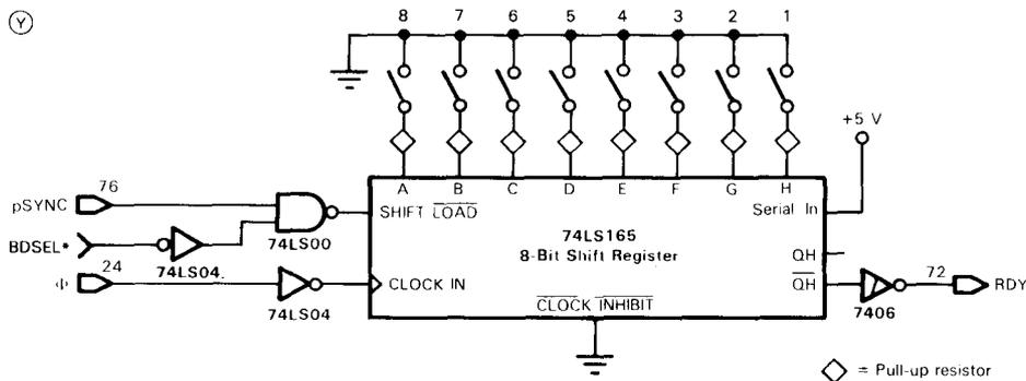
FIGURE 5-47. Circuit to Generate 0 to 8 Wait States
