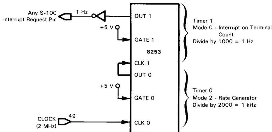
**FIGURE 14-7.** Timer Configuration for Interrupting Interval
