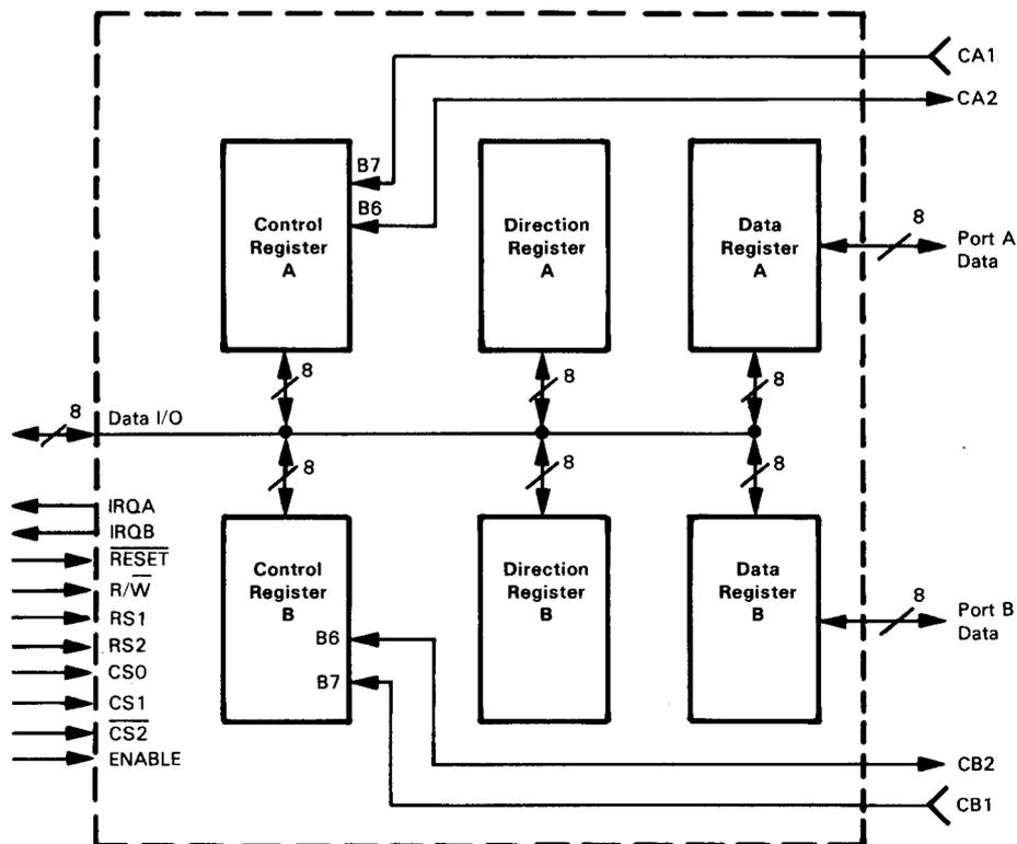
FIGURE 7-11. Functional Block Diagram of the MC6820 PIA
