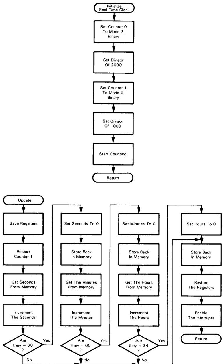
FIGURE 14-8. Flowchart for Real Time Clock Program
