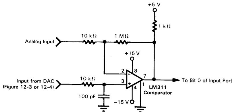
FIGURE 12-9. Added Circuitry For Ramp and Successive Approximation ADC
