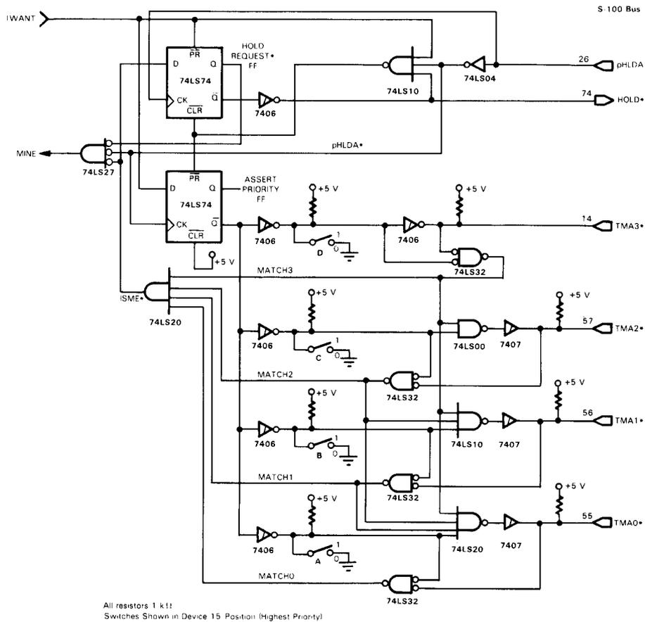
FIGURE 15-3. Arbitration Logic for S-100 TMA Controller
