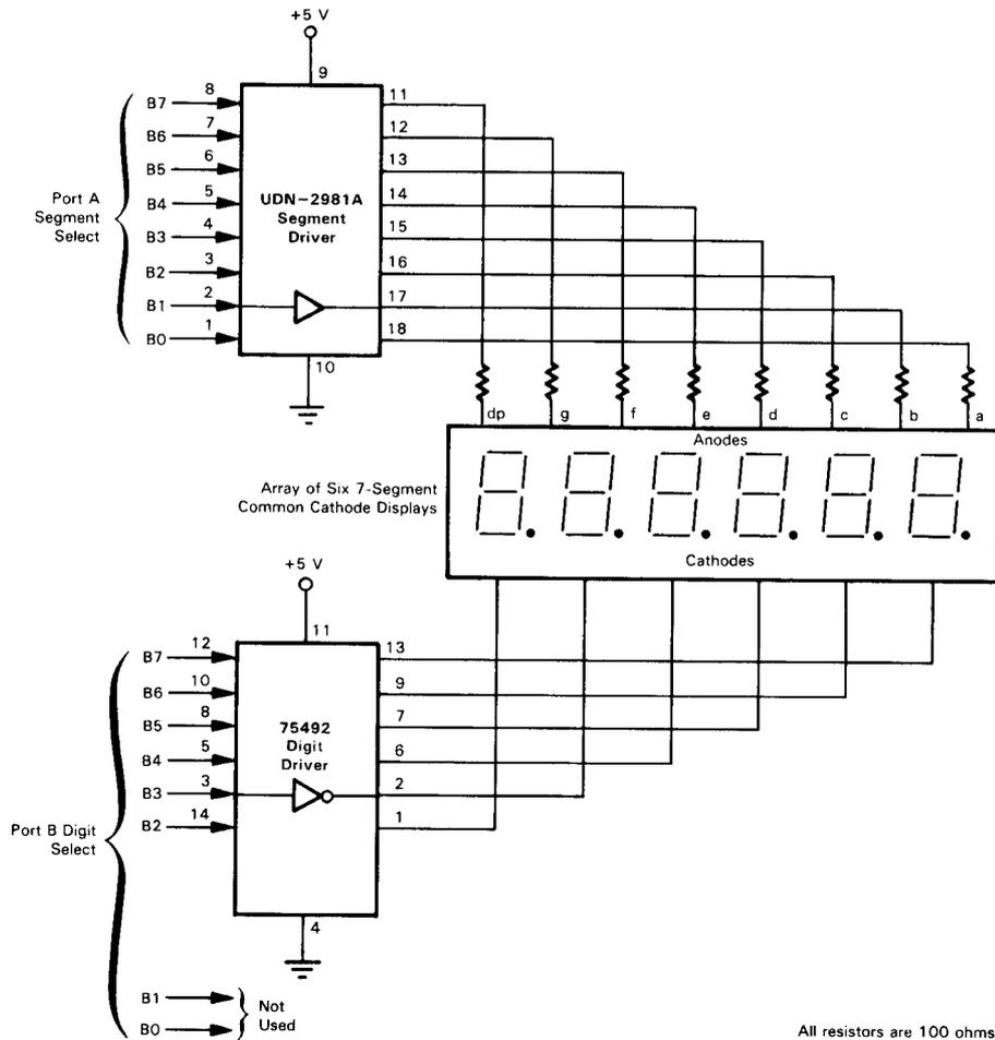
FIGURE 10-3. Wiring for a Multiplexed 6-Digit Display
