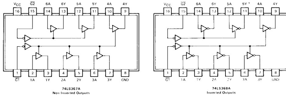
FIGURE 5-7. Hex Bus Drivers with Tri-State Outputs
