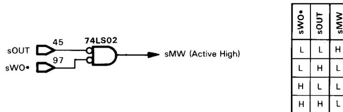
FIGURE 3-1. Circuit to Generate Status Memory Write Signal
