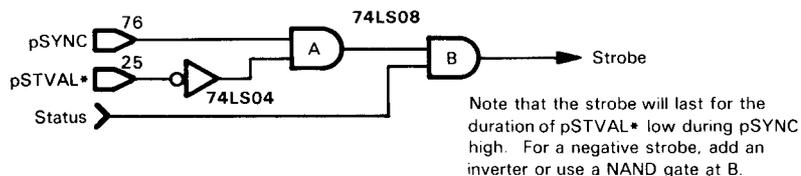
FIGURE 5-14. Circuit for Developing a Glitch-Free Strobe Signal
