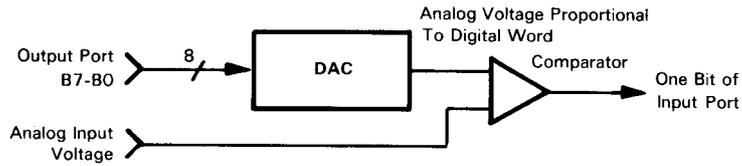
FIGURE 12-8. ADC System Where DAC Output is Compared Against Unknown Analog Input
