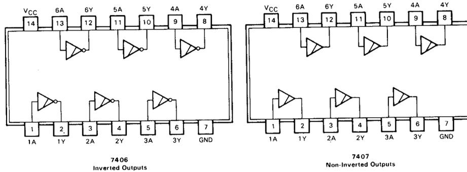
**FIGURE 5-9.** Hex Inverter Buffers/Drivers with Open Collector Outputs
