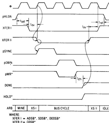
Figure 8. Bus transfer and single bus cycle.
