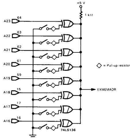
FIGURE 5-28. Extended Memory Address Decoder Circuit .
