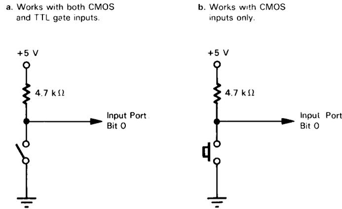
FIGURE 9-1. Connecting Switches to an Input Port
