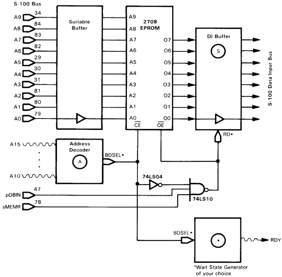
FIGURE 6-13. 1K x 8 of 2708-Type EPROM Interfaced to the S-100 Bus
