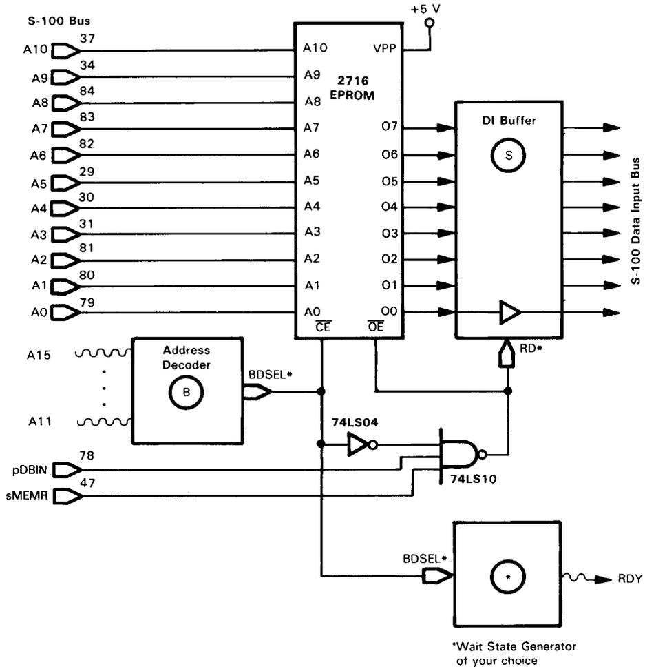
FIGURE 6-14. 2K x 8 of 2716-Type Memory Interfaced to the S-100 Bus
