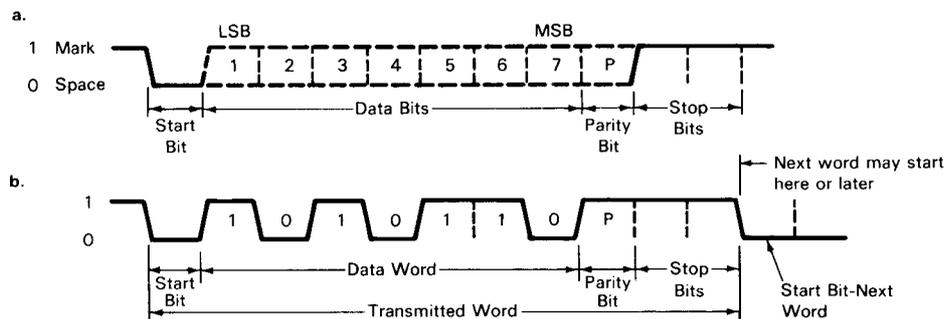
FIGURE 11-2. (a) Serial Transmission Format;
