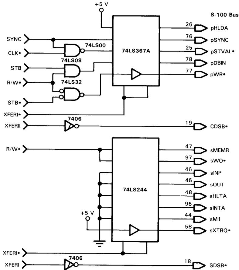
**FIGURE 15-11.** Control and Status Bus Logic for S-100 TMA Controller
