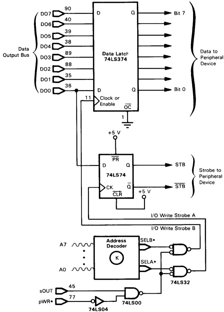
FIGURE 8-4. Latched Output Port with Handshaking Strobe
