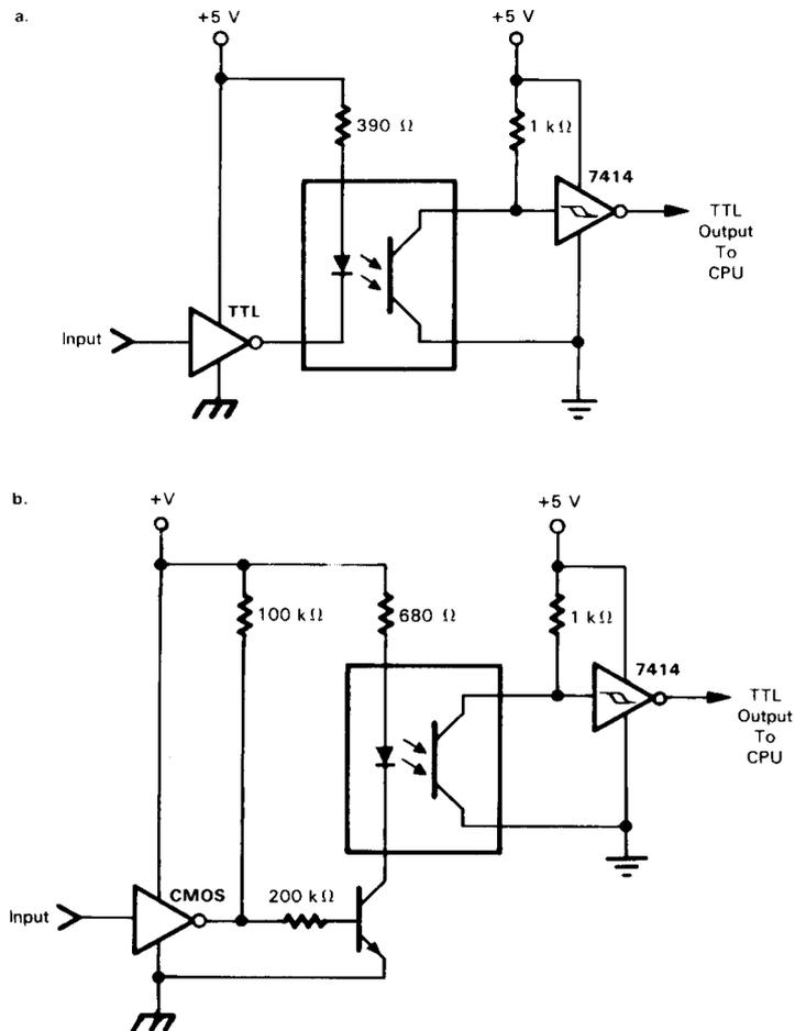
FIGURE 9-18. Isolating Logic Systems From the CPU
