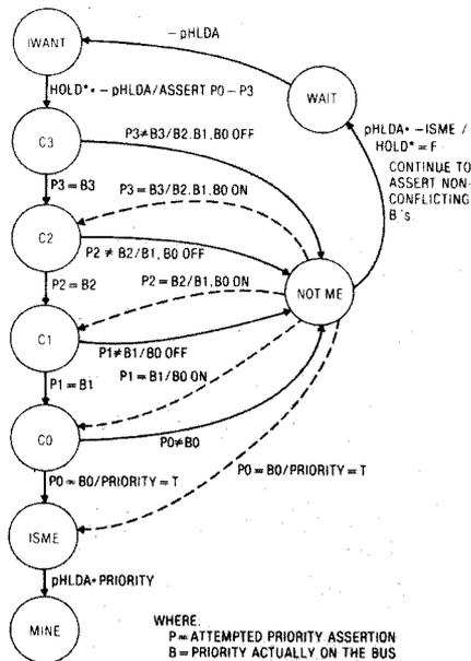
Note: This state diagram is conceptually correct, but this process is actually a parallel rather than a sequential one. Figure 9b shows suitable logic to implement such a parallel process.
