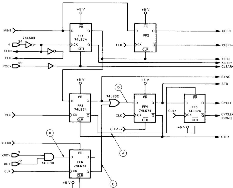
FIGURE 15-6. Timing Logic for S-100 TMA Controller
