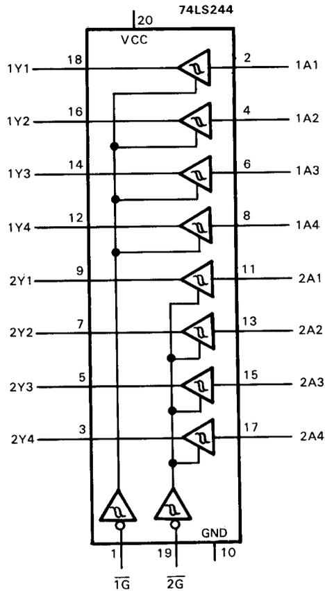
FIGURE 8-3. 74LS244 Logic Symbol with Pin Connections
