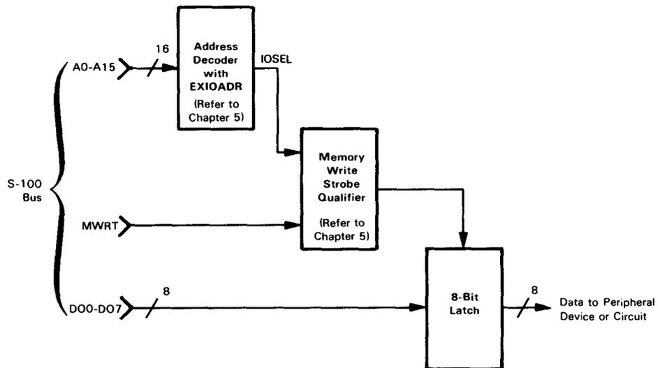
FIGURE 7-4. Block Diagram of a Memory-Mapped Output Port
