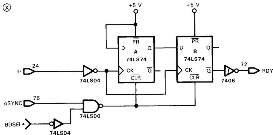
**FIGURE 5-46.** Circuit to Generate Two Wait States
