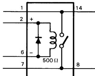
FIGURE 10-4. Pin-Out Diagram for Sigma 191TE1A2-5S Relay
