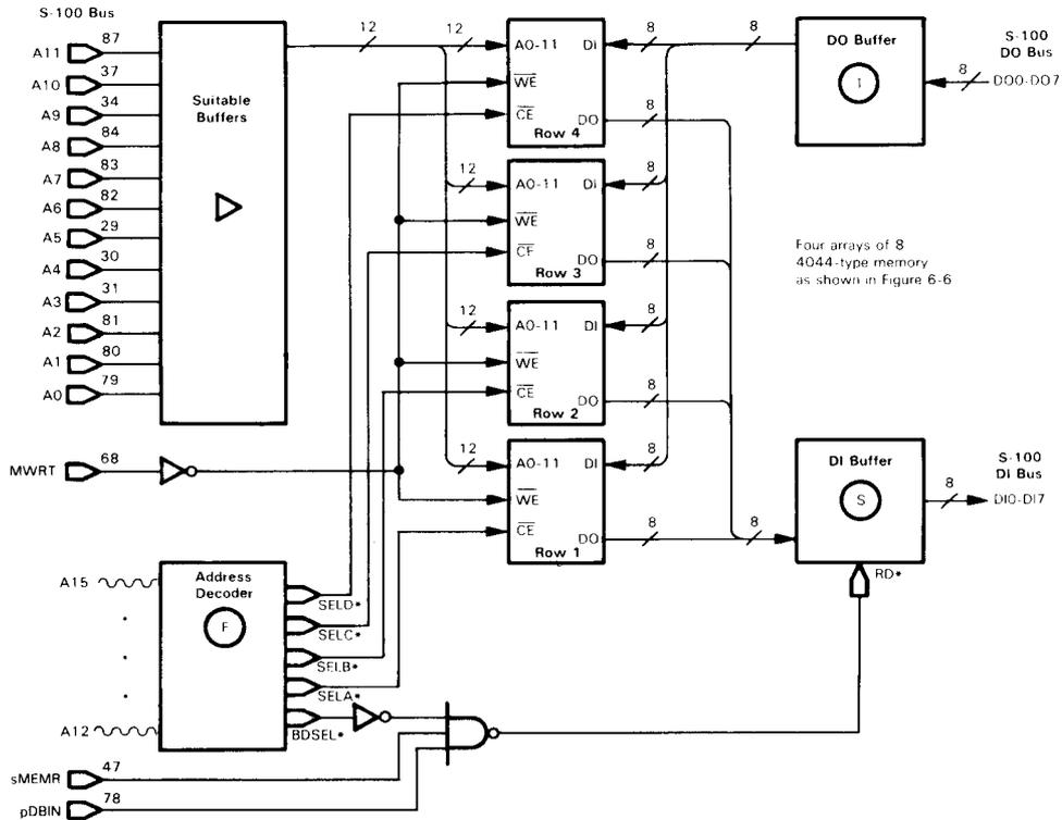
**FIGURE 6-10.** 16K × 8 of 4044-Type Memory Interfaced to the S-100 Bus
