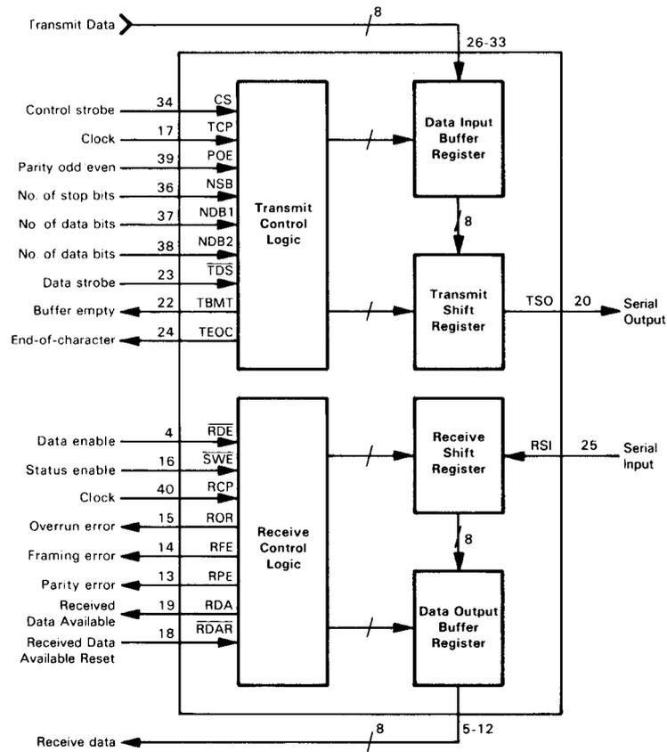
FIGURE 11-3. Block Diagram of the AY-5-1013A UART
