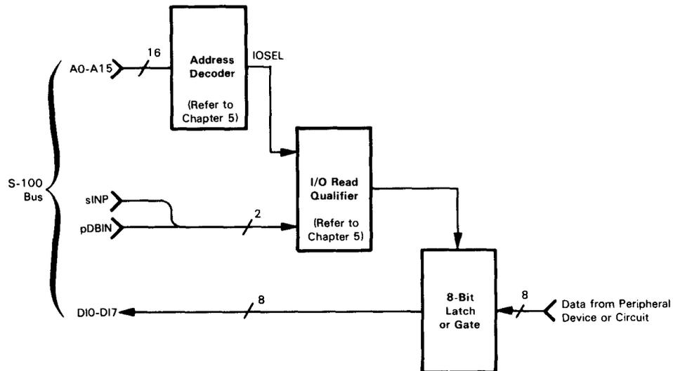
FIGURE 7-3. Block Diagram of a Typical Input Port
