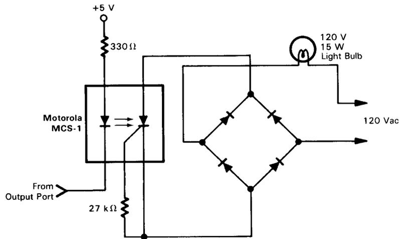
**FIGURE 10-7.** AC Control Using an Opto-Coupler/SCR
