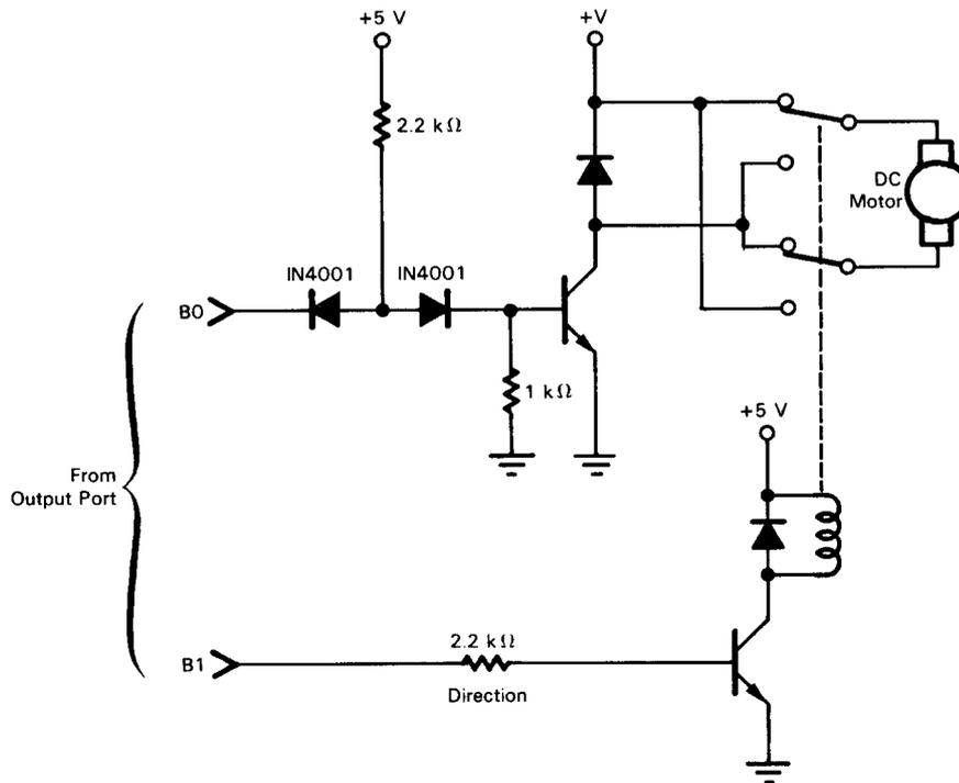
**FIGURE 10-12.** Simple Low-Power DC Motor Interface Circuit
