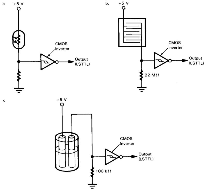
Note: All inverters are CMOS Schmitt Trigger Gates
