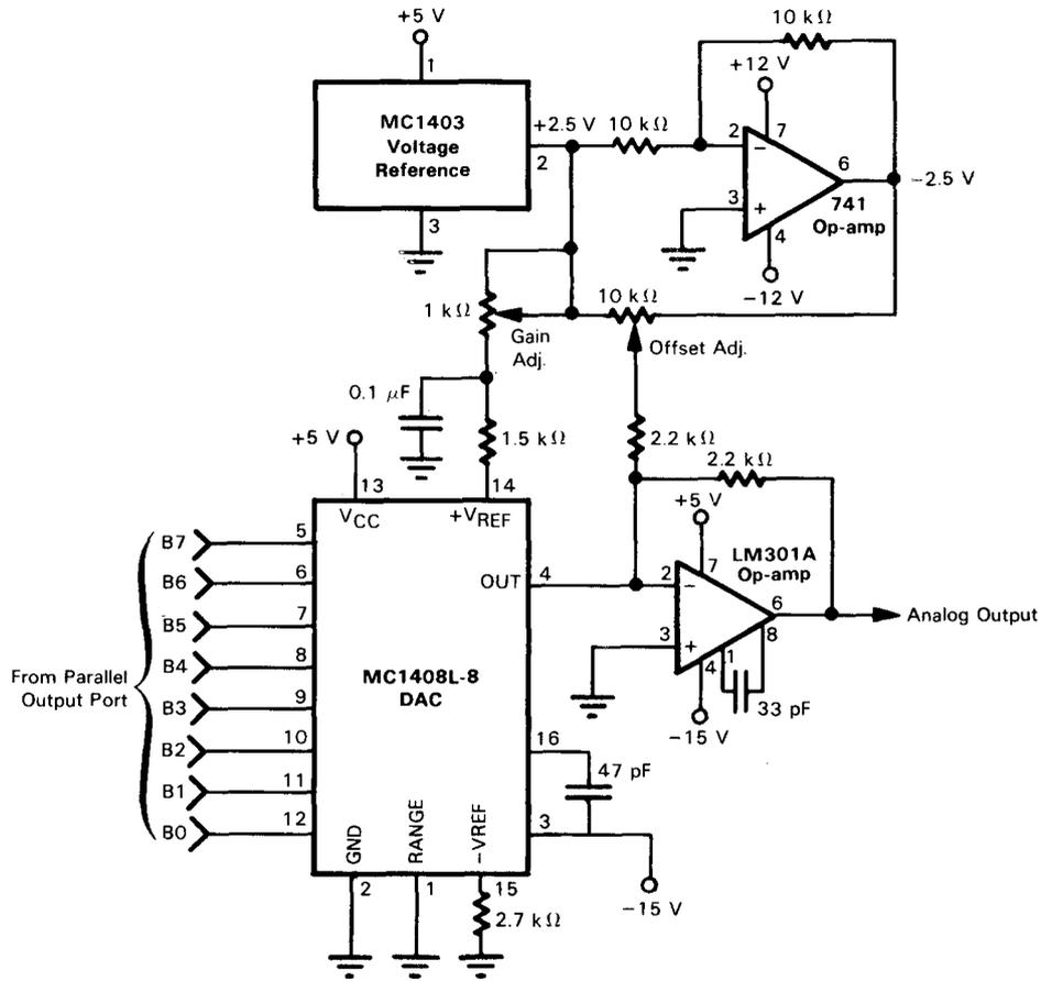
FIGURE 12-4. An Improved 1408 DAC Circuit
