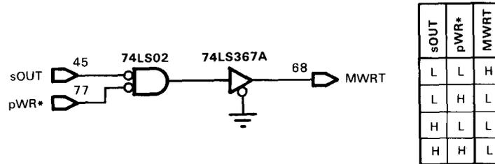
**FIGURE 3-3.** Circuit to Generate MWRT
