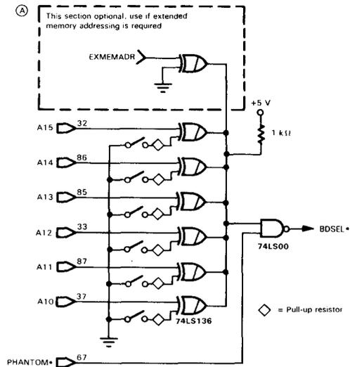
**FIGURE 5-19.** Memory Address Decoder for One 1K Block
