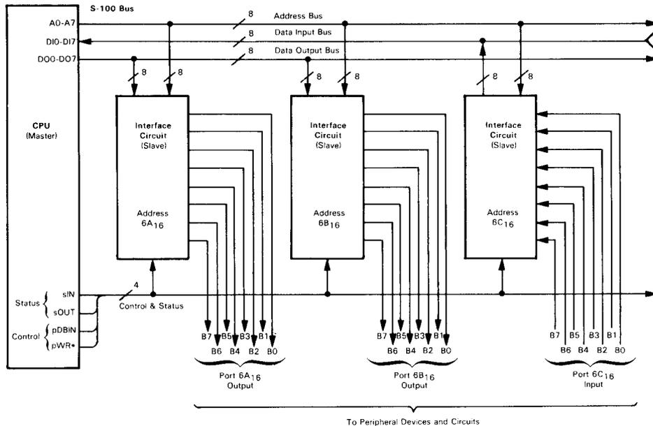
**FIGURE 7-1.** Block Diagram of CPU With Two Output Ports ( $6A_{16}$  &  $6B_{16}$ ) and One Input Port ( $6C_{16}$ )
