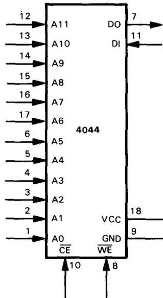
FIGURE 6-5. 4044 Logic Symbol with Pin Connections
