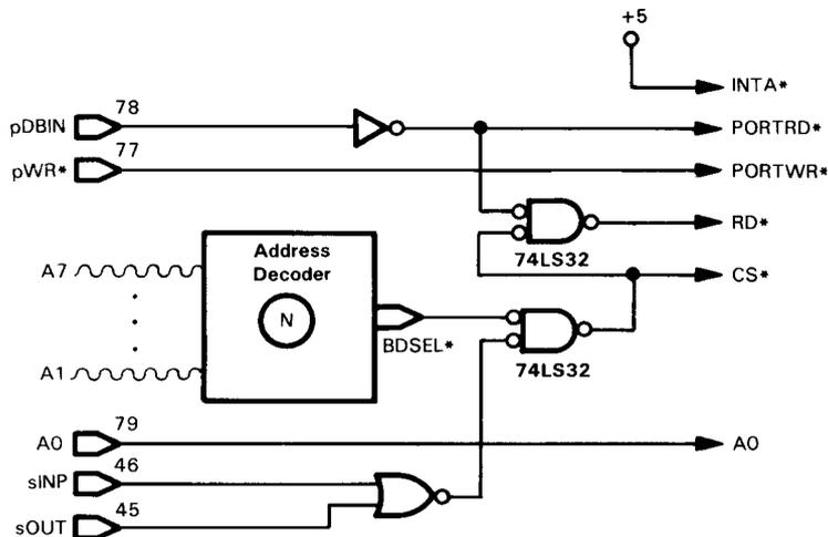
**FIGURE 13-11.** Alternative S-100 Interface for 8259A Using Polled Mode (See Figure 13-10)
