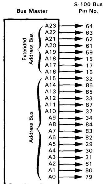
**FIGURE 2-4.** The S-100 Address and Extended Address Bus
