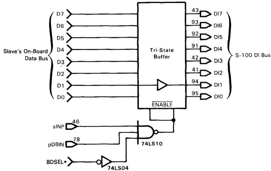
FIGURE 5-39. I/O Read Strobe Qualifier Circuit
