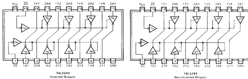
FIGURE 5-8. Octal Bus Drivers with Tri-State Outputs
