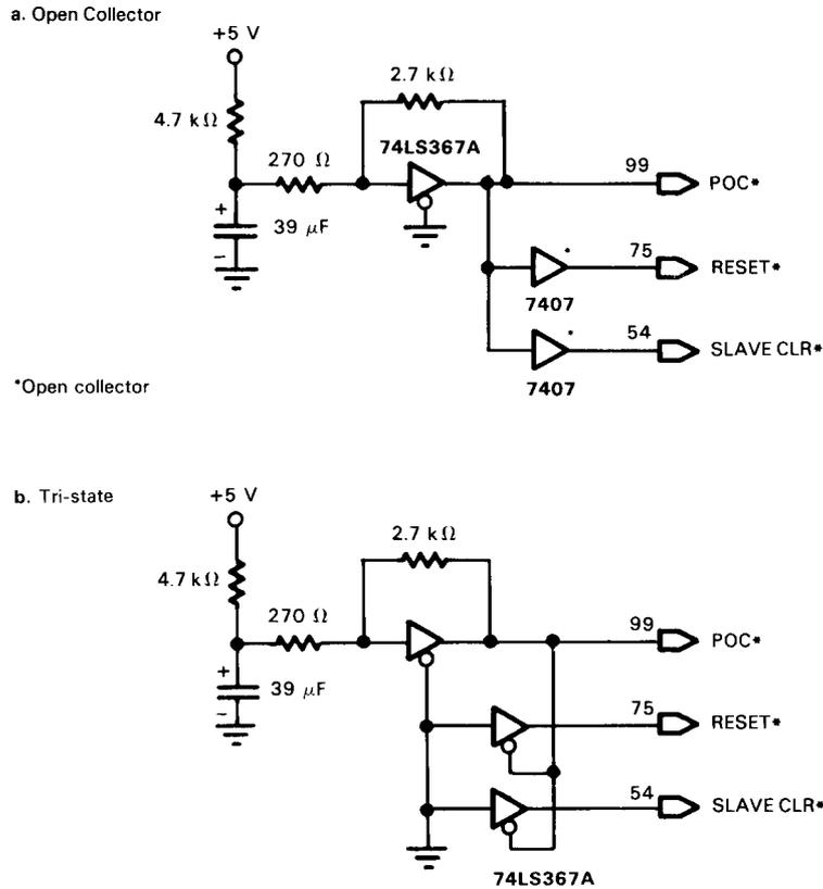
**FIGURE 3-4.** Two Circuits That Correctly Generate POC\*
