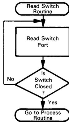
FIGURE 9-2. Read Switch Routine Flowchart
