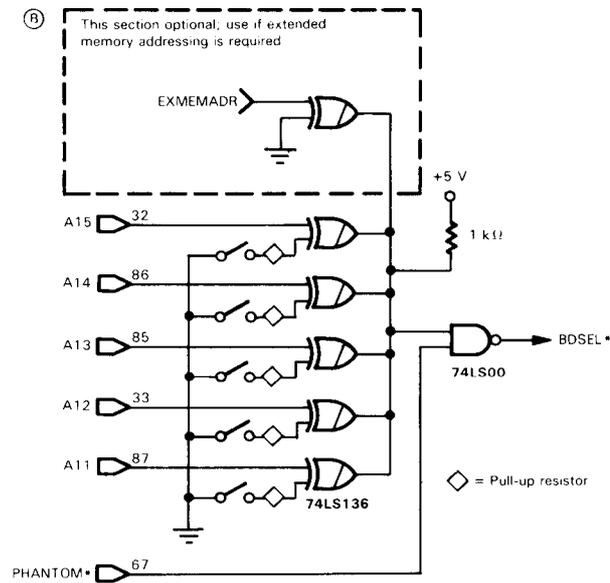
FIGURE 5-20. Memory Address Decoder for One 2K Block
