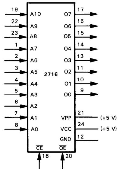
FIGURE 6-12. 2716 Logic Symbol with Pin Connections
