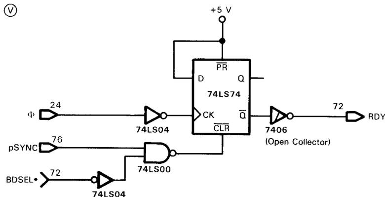
FIGURE 5-45. Circuit to Generate One Wait State
