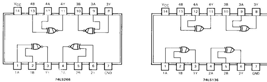
FIGURE 5-15. Quad Exclusive-NOR and -OR Gates with Open Collector Outputs
