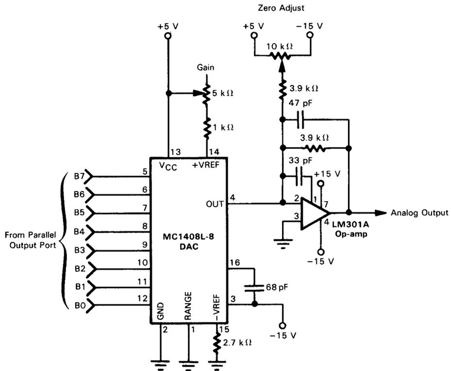
FIGURE 12-3. A Simple 1408 DAC Circuit
