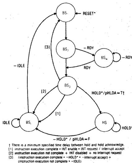
Figure 1. Permanent master state diagram.
