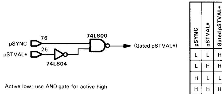
**FIGURE 3-2.** Circuit That Gates pSTVAL\* with pSYNC
