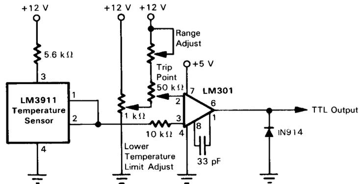
FIGURE 9-13. Precision Temperature Sensing Circuit
