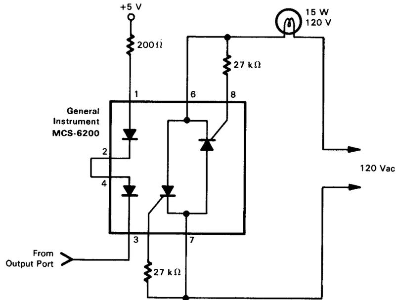
FIGURE 10-8. AC Control Using an Opto-Coupler/Dual SCR
