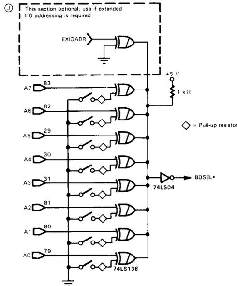
FIGURE 5-29. I/O Address Decoder for One I/O Port
