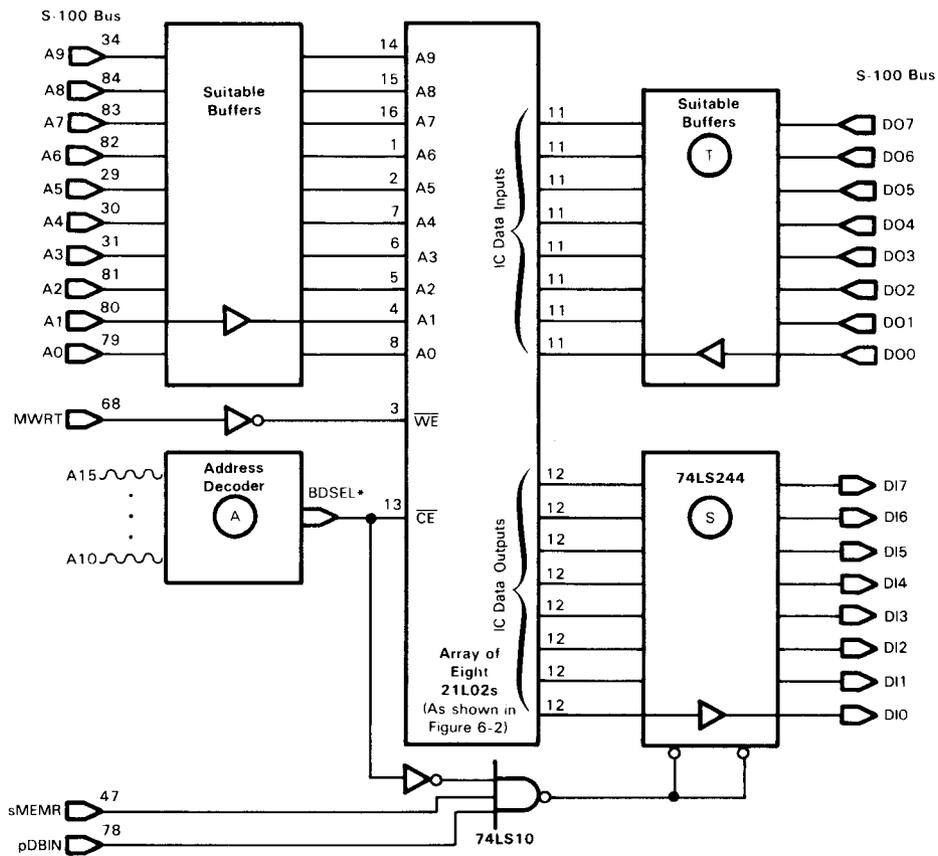
**FIGURE 6-8.**  $1K \times 8$  of 21L02-Type Memory Interfaced to the S-100 Bus
