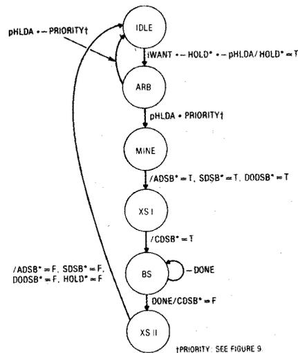
Figure 7. Bus transfer state diagram.
