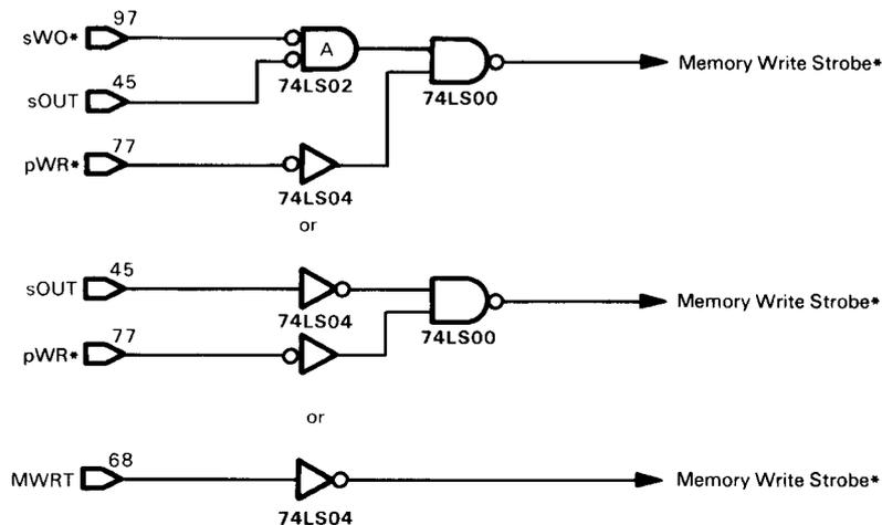
FIGURE 5-40. Memory Write Strobe Qualifier Circuits
