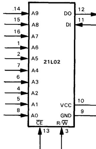
FIGURE 6-1. 21L02 Logic Symbol with Pin Connections
