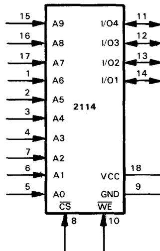
FIGURE 6-3. 2114 Logic Symbol with Pin Connections
