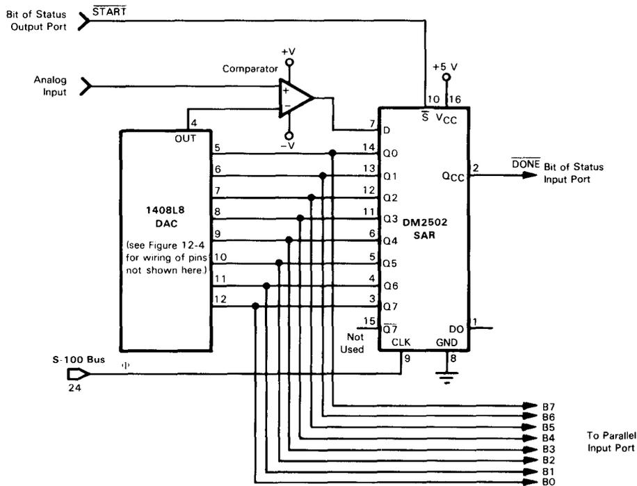
FIGURE 12-10. ADC Using Hardware Successive Approximation Register
