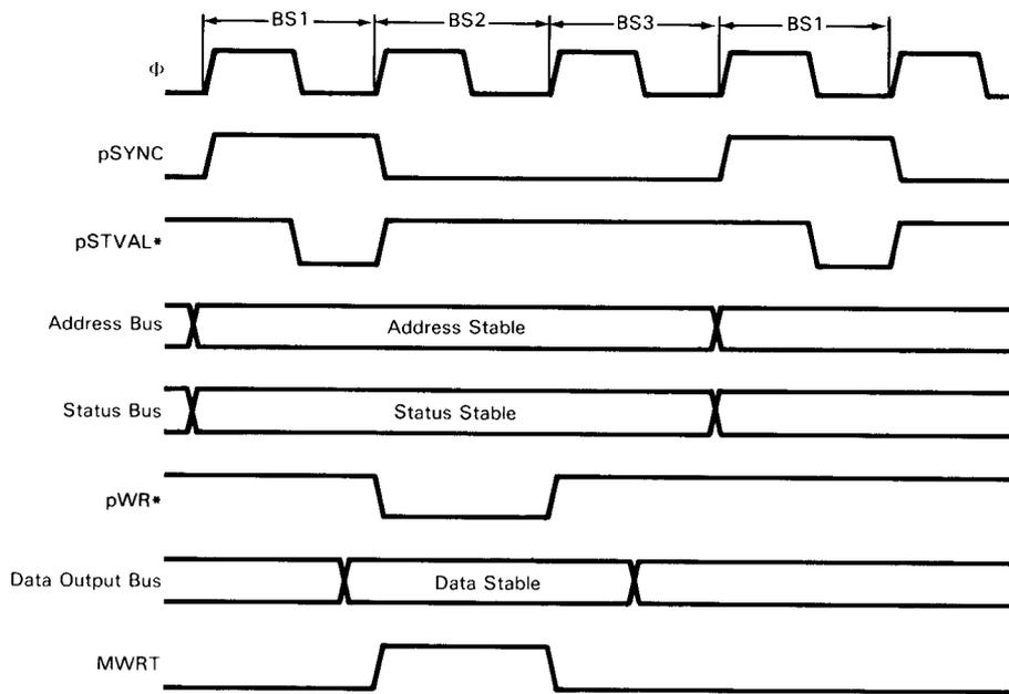
**FIGURE 4-4.** S-100 Bus Write Cycle
