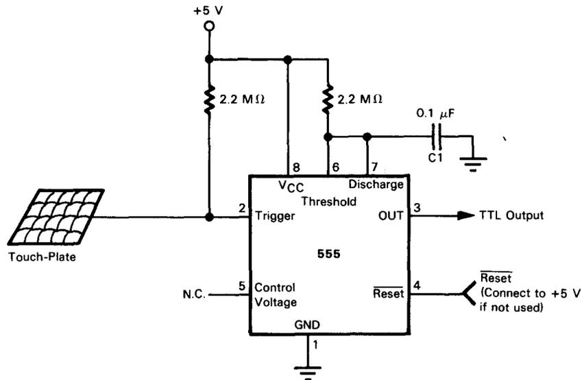
FIGURE 9-14. A Touch-Plate Sensing Circuit
