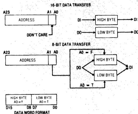
Figure 5. 8/16-bit address and data usage.
