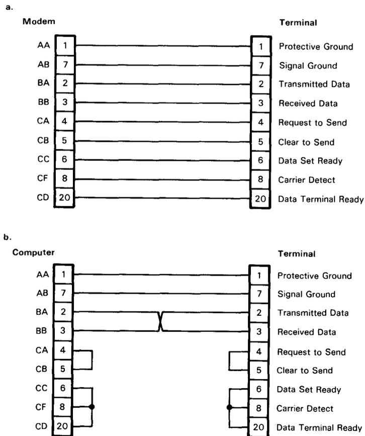
FIGURE 11-9. RS-232 Cable Wiring; (a) Modem-Terminal, (b) Computer-Terminal
