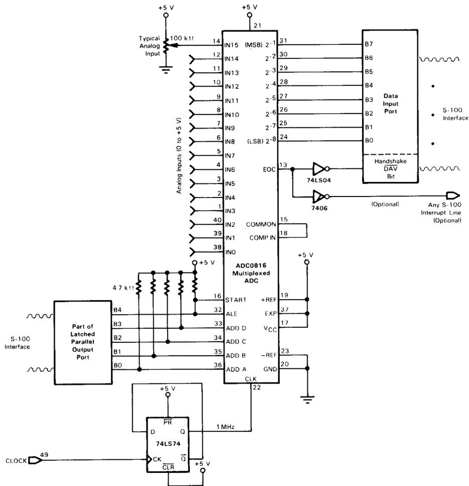
FIGURE 12-11. S-100 Interface of 16 Channel ADC Through Parallel Channels
