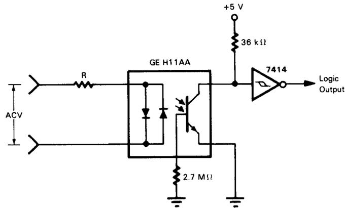
FIGURE 9-17. AC Voltage Sensor Circuit
