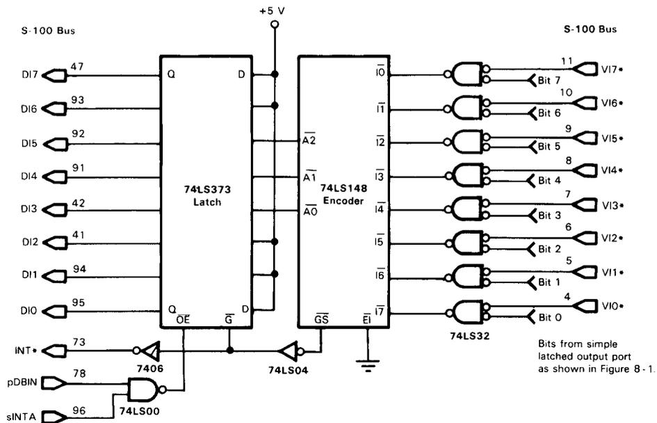
FIGURE 13-7. Simple Priority Interrupt Controller with Full Masking
