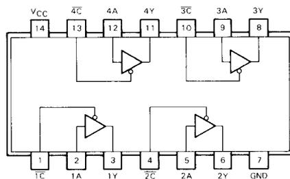
**FIGURE 5-5.** 74LS125A Quadruple Bus Drivers with Tri-State Outputs
