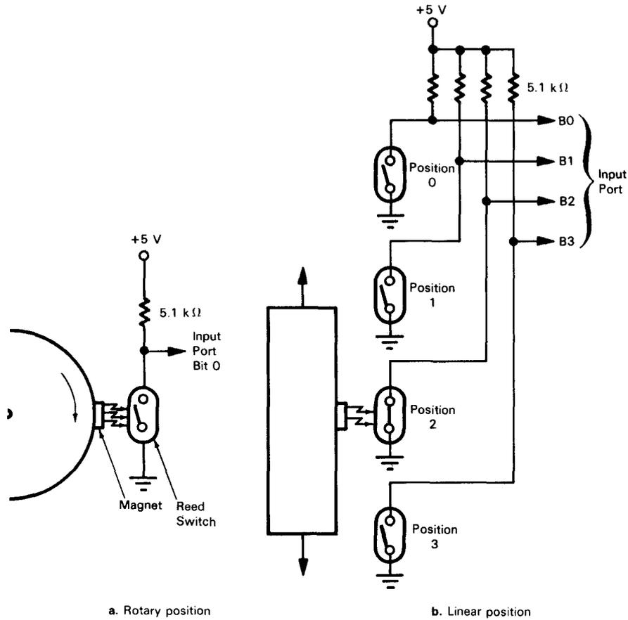
FIGURE 9-5. Determining Position With Magnetically Operated Switches
