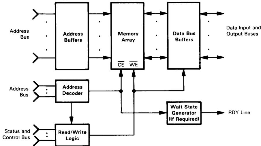
**FIGURE 6-7.** Block Diagram of Typical S-100 Memory Board
