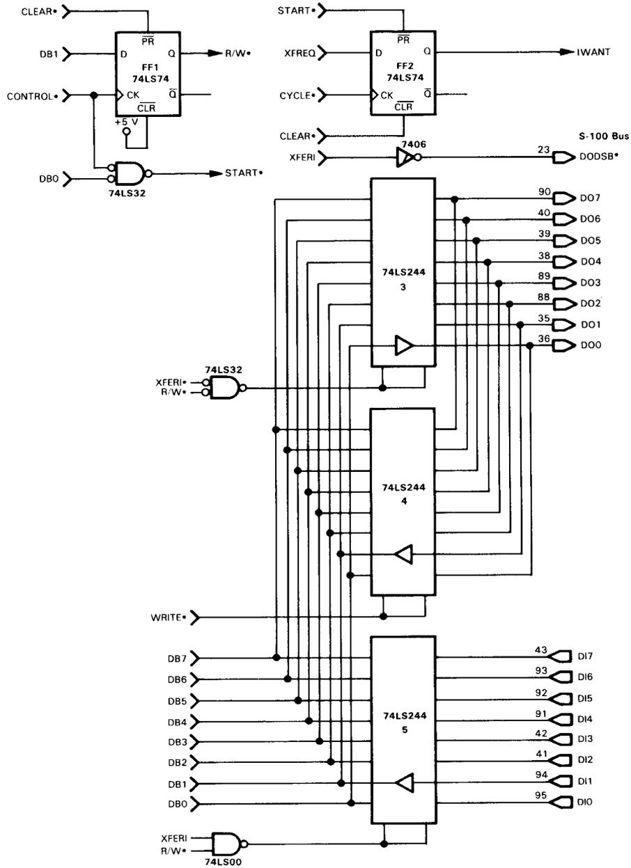
FIGURE 15-10. Data Bus Control Logic; Start Pulse and Direction Bit Logic
