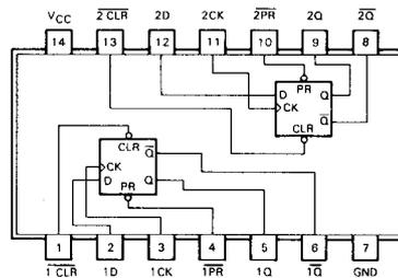
FIGURE 7-6. 74LS74 Dual D-Type Latch
