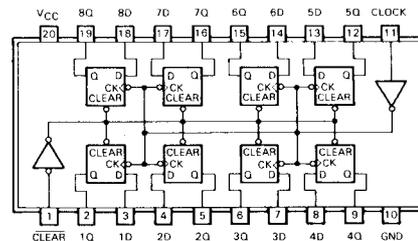
FIGURE 7-8. 74LS273 Octal D-Type Latch
