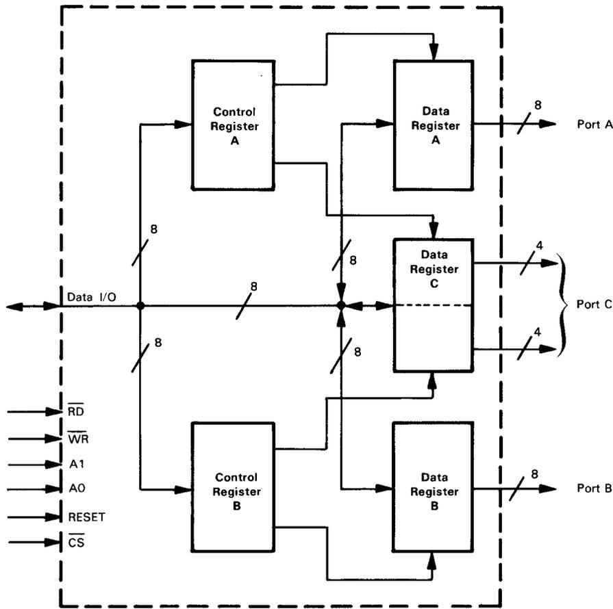
FIGURE 7-12. Functional Block Diagram of the 8255 PPI
