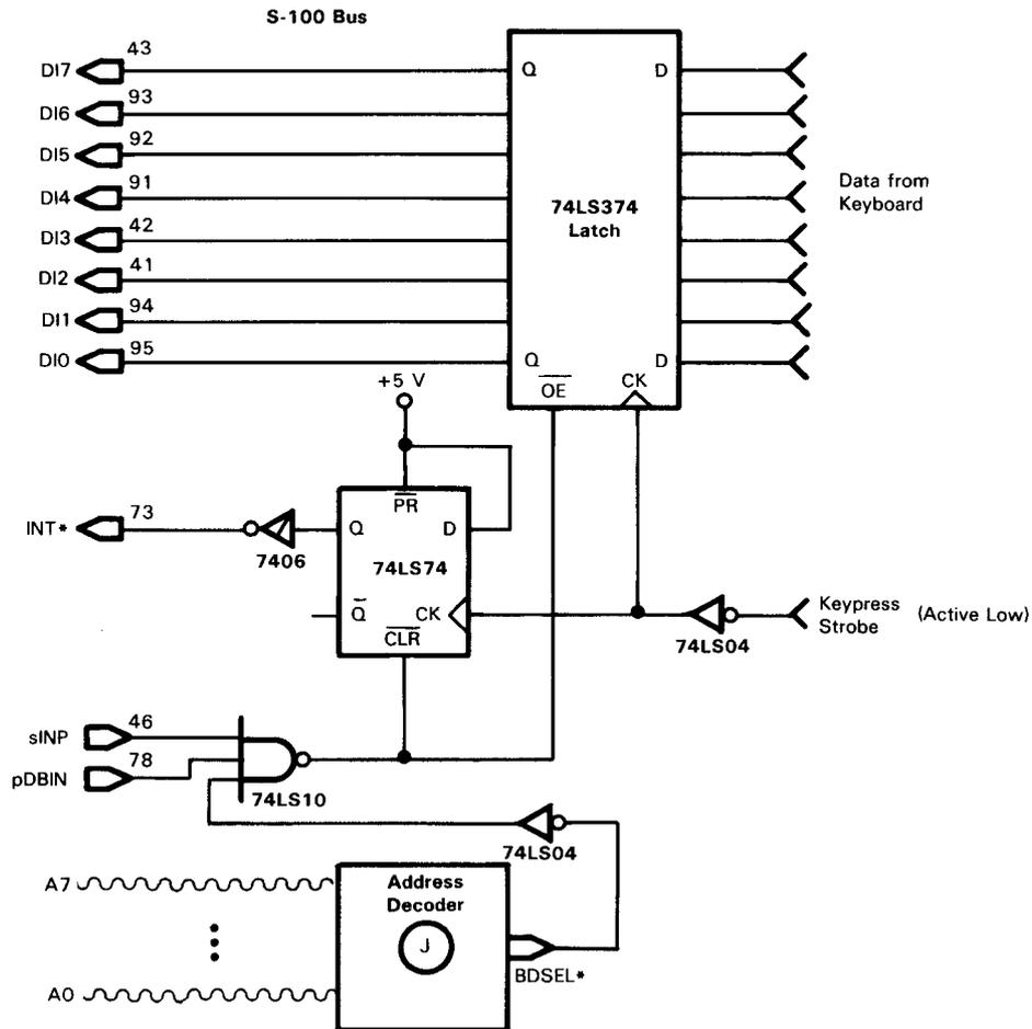
FIGURE 13-3. Simple Single Interrupt Circuit
