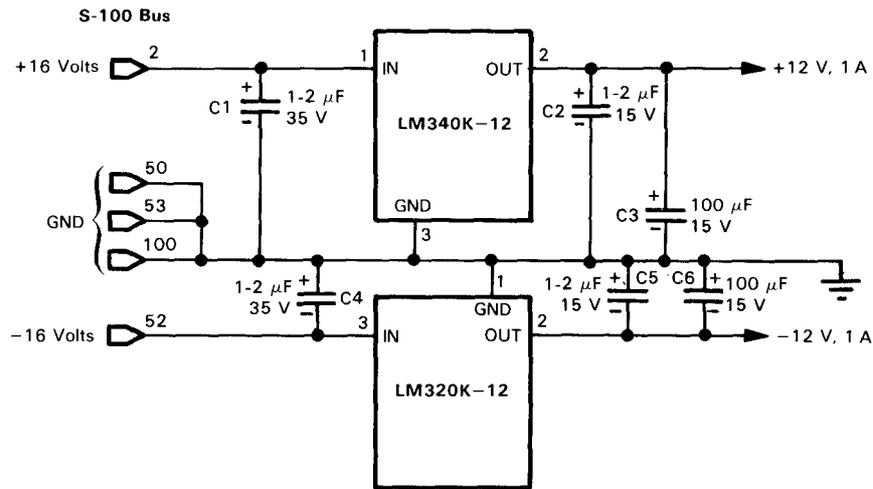
FIGURE 2-8. Typical +12 Volt and -12 Volt Regulator Circuits
