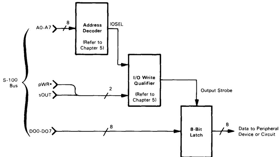
FIGURE 7-2. Block Diagram of a Typical Output Port
