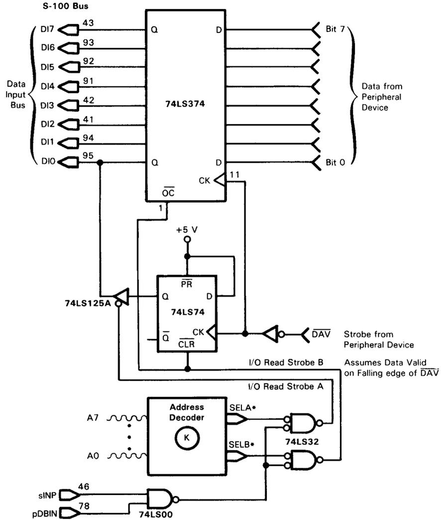
FIGURE 8-8. Latched Input Port with  $\overline{\text{DAV}}$  Strobe
