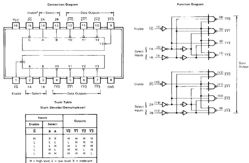
FIGURE 5-18b. Dual 2- to 4-Line Decoder
