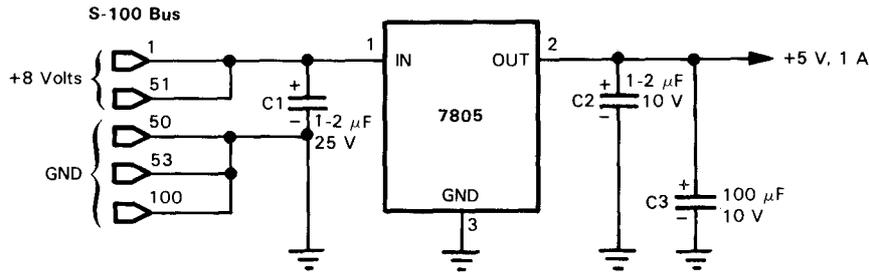
FIGURE 2-7. Typical +5 Volt, 1 A Regulator Circuit
