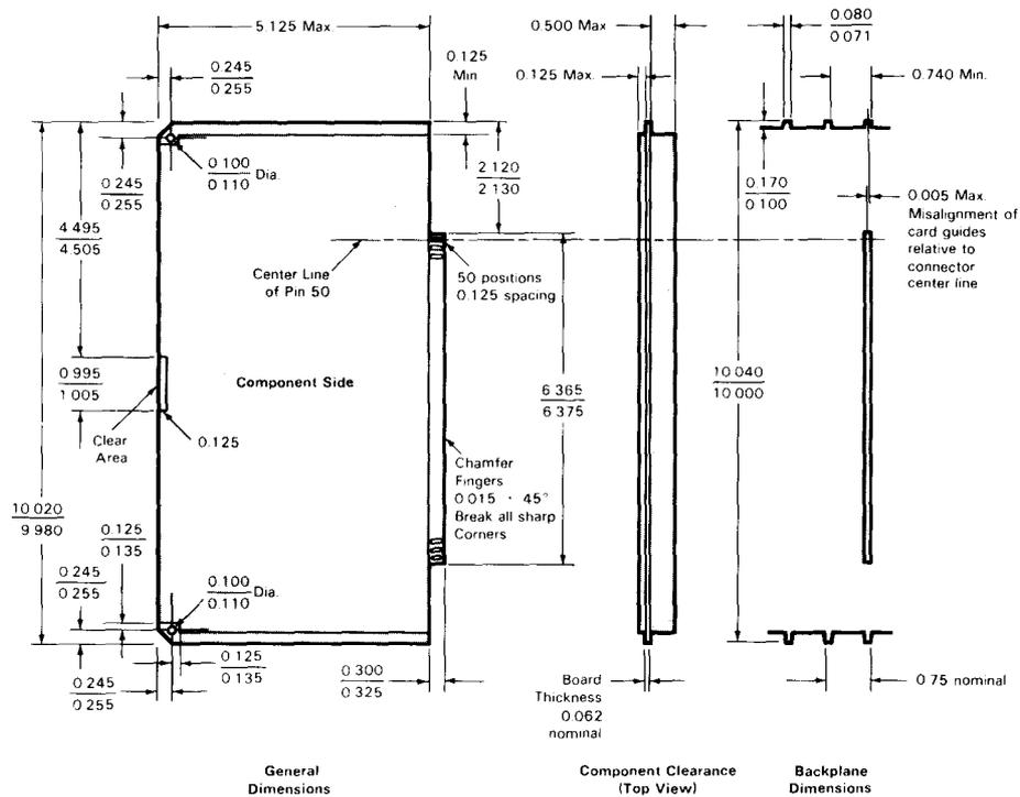
**FIGURE 2-1.** S-100 Plug-In Board Mechanical Specifications
