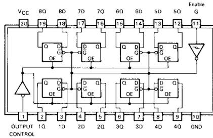
FIGURE 7-9. 74LS374 Octal D-Type Latch
