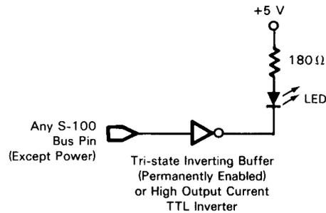
**FIGURE 16-1.** Adding LEDs to Monitor S-100 Signal Lines
