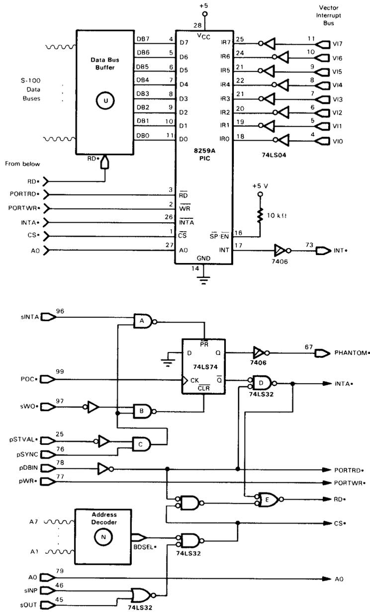
FIGURE 13-10. Priority Interrupt System Using the 8259A
