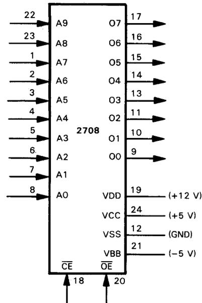
FIGURE 6-11. 2708 Logic Symbol with Pin Connections
