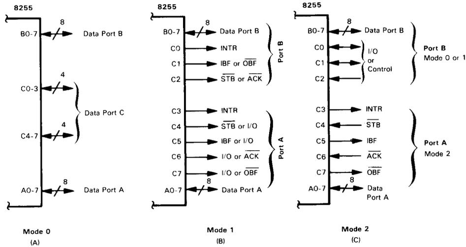
FIGURE 7-13. The Three Modes of Operation of the 8255
