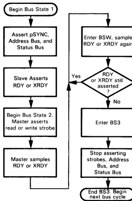
FIGURE 4-6. Bus Cycle with Wait State Flowchart
