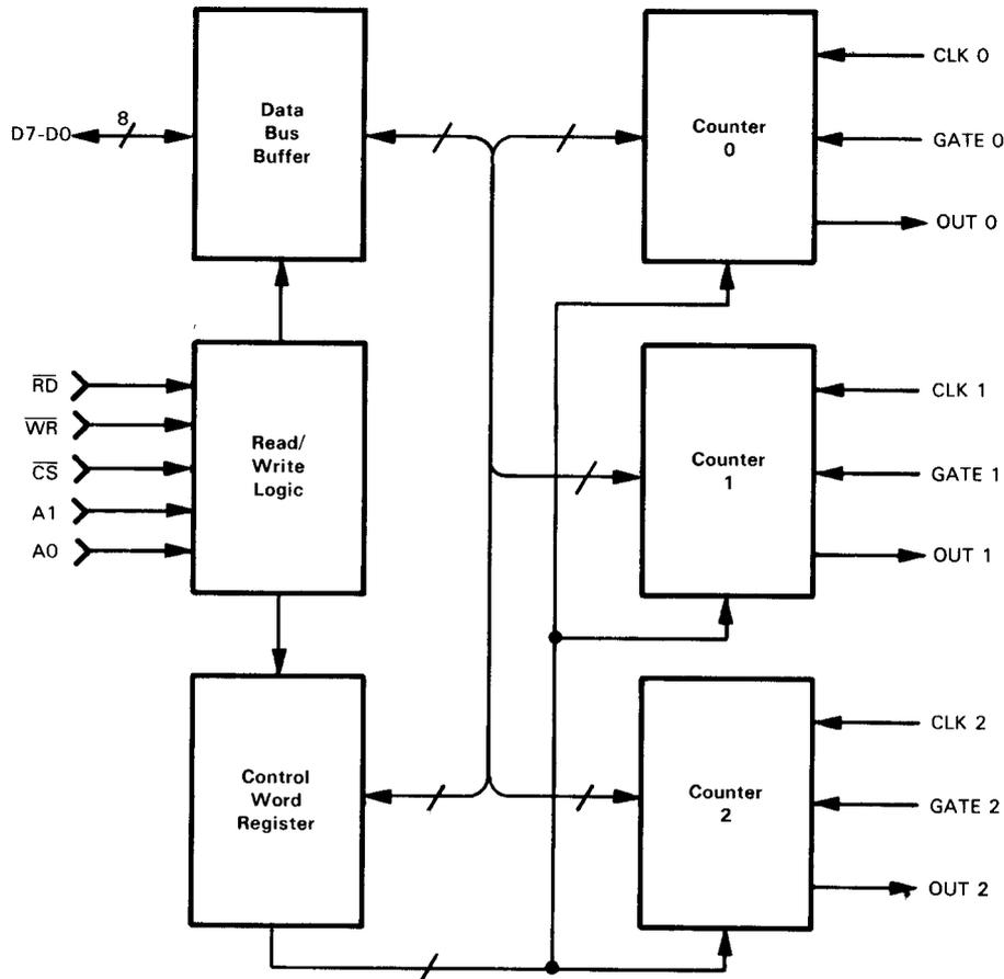
FIGURE 14-1. Block Diagram of 8253 Programmable Interval Timer
