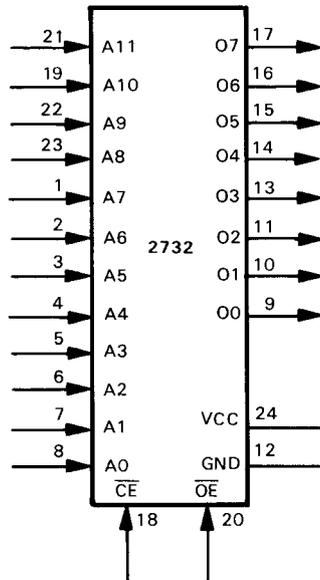
FIGURE 6-17. 2732 Logic Symbol with Pin Connections
