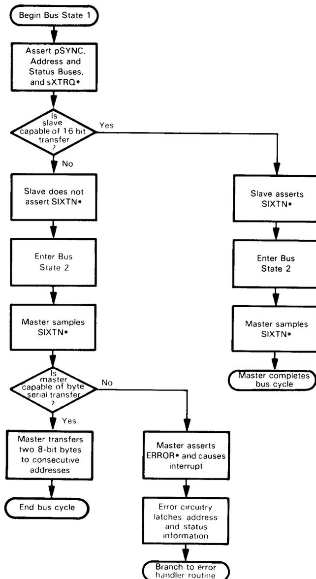
FIGURE 4-8. Sixteen-Bit Data Transfer Flowchart
