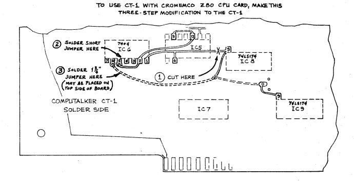
Note that the above hardware modification has been factory installed on all boards with serial numbers 431 and higher. It is compatible with both 8080 and Z-80 processors.
