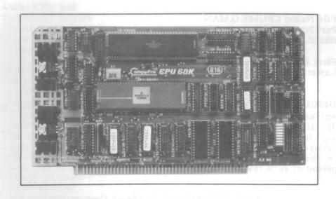
16 BIT 68000 WITH PROVISIONS FOR MMU AND UP TO 16K BYTES OF ROM CLOCK RATES TO 10 MHz
